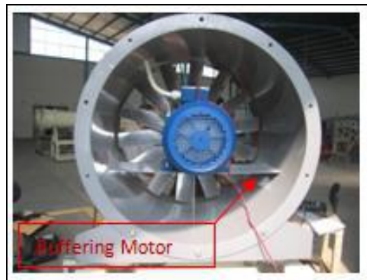
Fig.9: Buffering of axial fan engine that needs to be reinforced.
