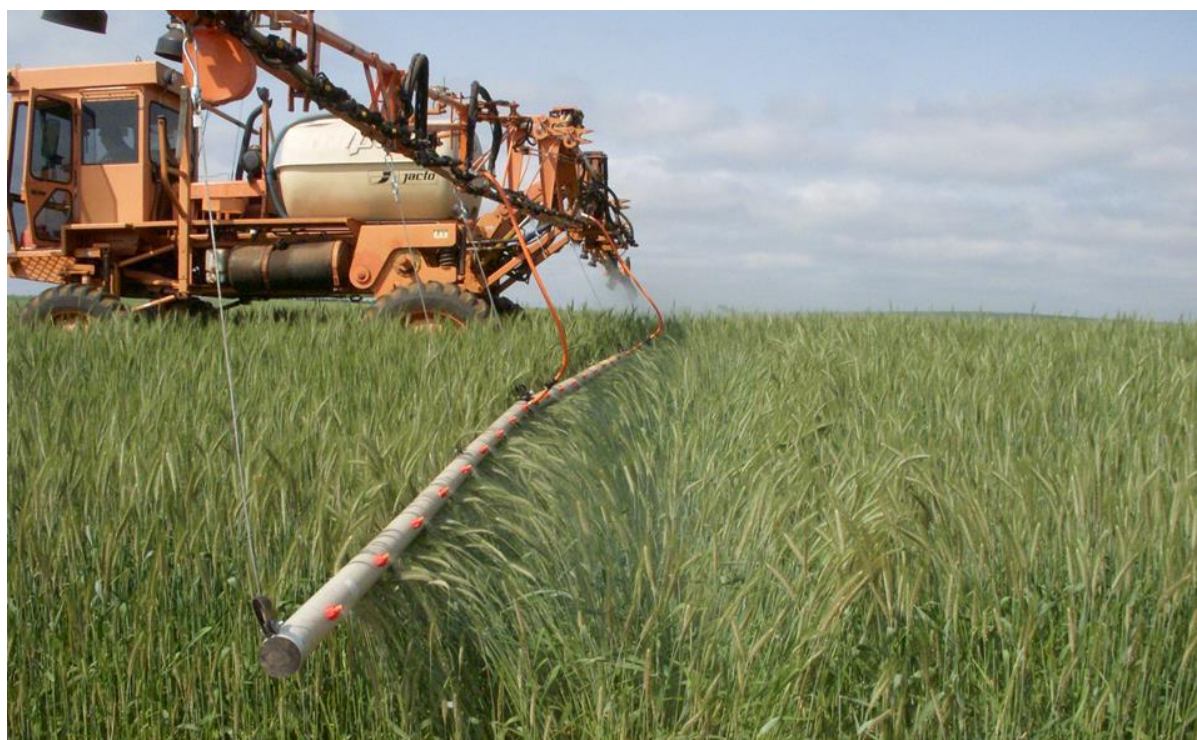
Fig.1: Trailing boom (kit alvo®) coupled to a traditional sprayer (Image: Willy Schnepfer Junior).
