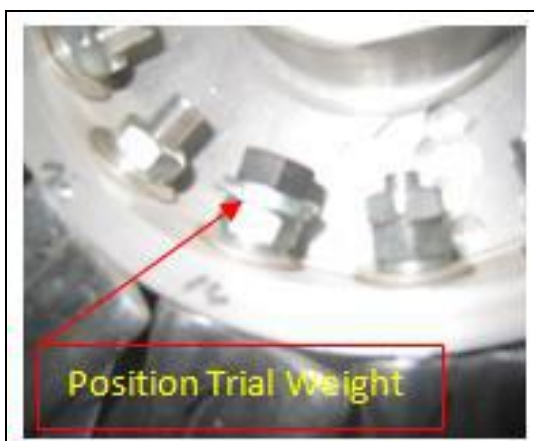
Fig.5: Location of trial weight on blade no. 14 at a hub axial fan engine.
